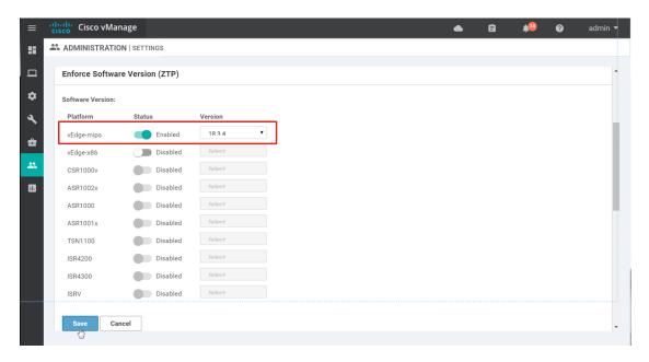
Br4-we2 is installed into the network. It is a vEdge 1000 and its ZTP port, ge0/0, is plugged into the Internet transport. It is assumed that br4-we2 is at factory defaults, and is currently running 17.2.7 software.
