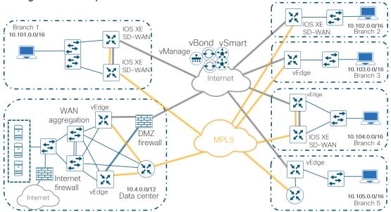
In this topology, there is one data center and five remote sites. The transports shown are one MPLS and one Internet service provider. The SD-WAN controllers are deployed using Cisco's cloud-managed service and reachable via the Internet transport. There is one vManage, one vSmart controller, and one vBond orchestrator on the U.S. West Coast, and there is one vSmart controller and one vBond orchestrator on the U.S. East Coast.
