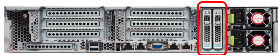
Currently Shipping UCS C240 M5 Rear View 2 boot drives option
